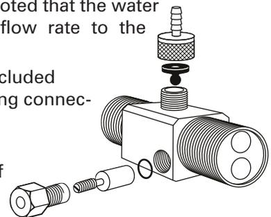
**The Dema 204B Air Injector** - This optional injector is constructed of solid brass with 1/2" Female threads and features a flow range for effective air draw of 2.9 - 9.5 GPM. While this air injector achieves air draws at lower flow rates, it should be noted once again that you cannot reduce the water flow rate below the backwash rate of your equipment.
